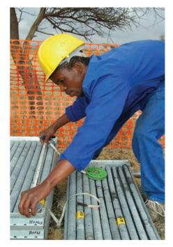
Samples of rock from the exploratory drilling being measured before going for analysis
