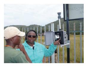
Monitoring air quality, March 2009. Small dust particles can cause serious breathing problems. This PM10 monitor measures dust particles that are less than one tenth of a millimetre in size. Wesizwe has to keep the dust produced by its activities to a minimum.
