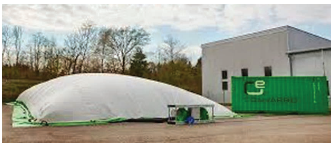
FIGURE 24: Pilot-scale Convaero Bio-Dry plant
