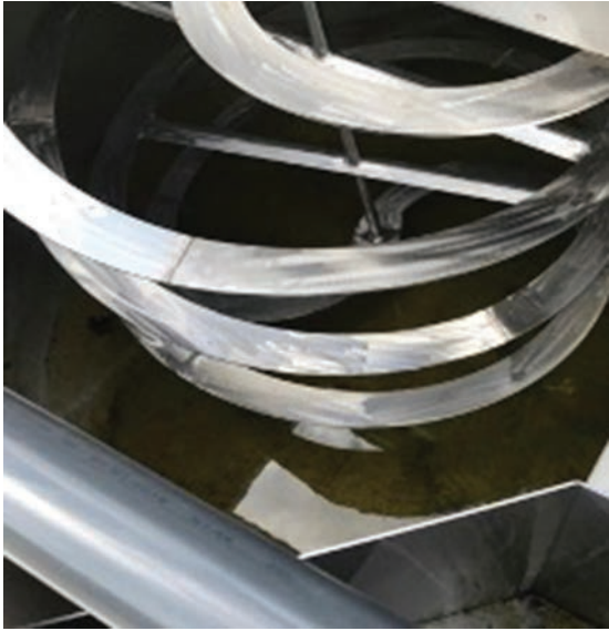
FIGURE 18: bioQUBE receiving tank mixer
