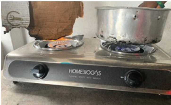
Testing of double burner of 7.0 unit to confirm flame
