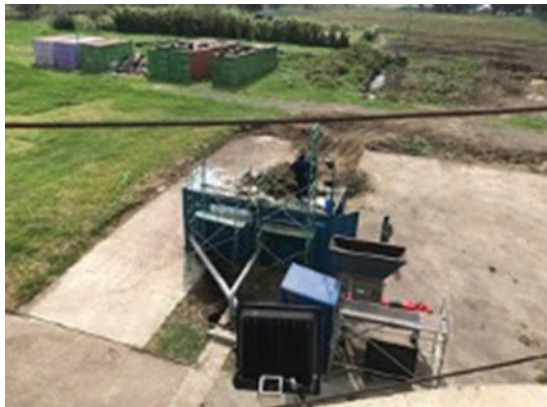
FIGURE 37: Feeding macerated rose stem and leaf waste into system
