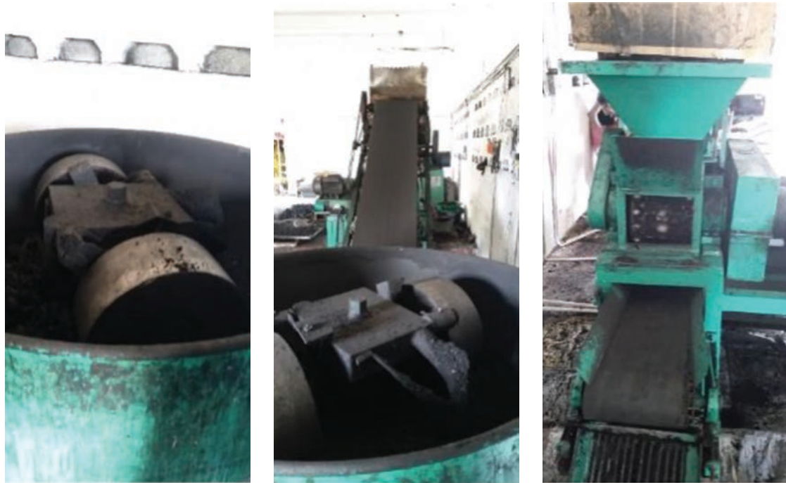
From left to right: shredder, conveyor belt and mold
