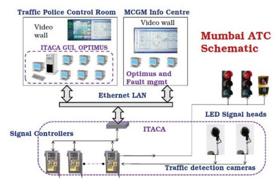
Figure 2: Schematic Representation of the deployed ATC System
